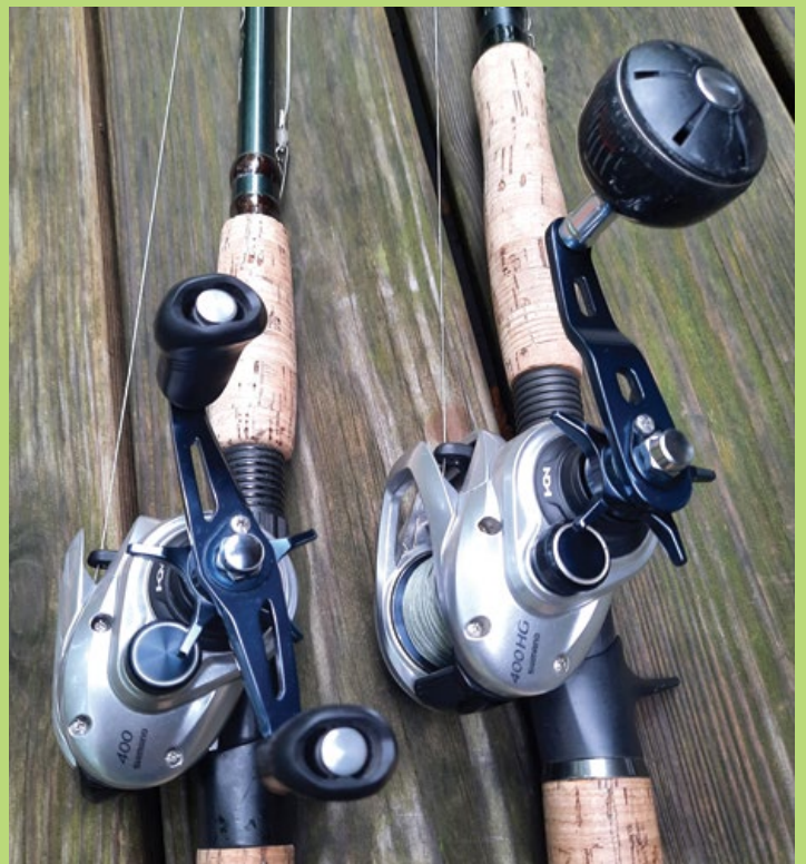
Retrieve speed and angler fatigue should be considered when selecting a reel. The model 400 (left—5.8:1 gear ratio, 30 IPT) recovers a hard-pulling lure easier than the 400HG (right—7.6:1, 40 IPT). However, the 400HG retrieves lighter lures faster.
