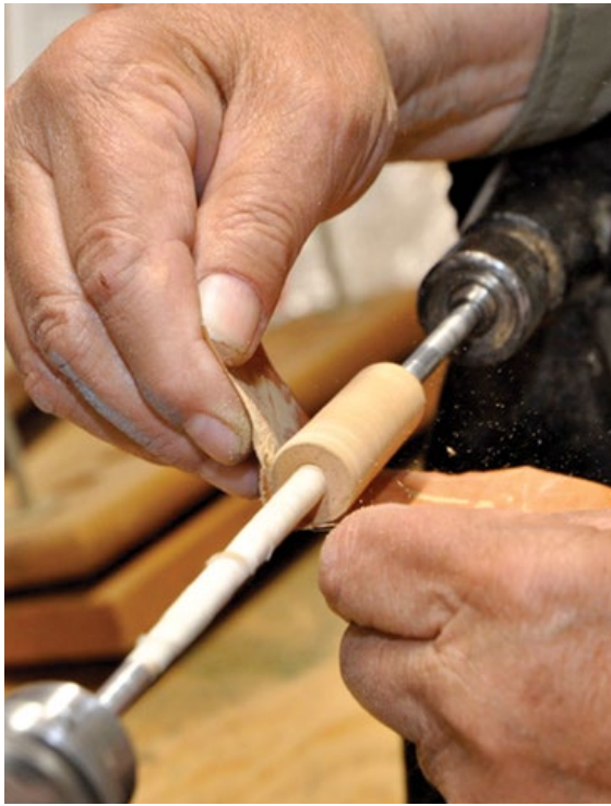
Sanding a piece of cork to make a custom handle.
