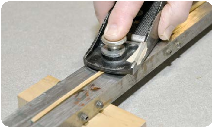
Art Weiler planes a bamboo section held in the steel form he built. Measurements of tapers from original bamboo rod makers are used to manufacture his reproduction fly rods. Set screws on both sides of the jig allow precise adjustments.
