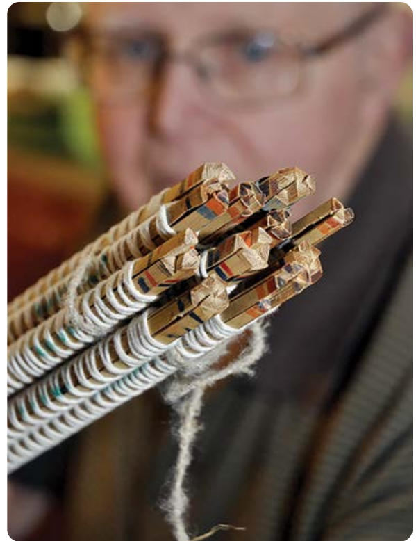
These bundled pieces of split bamboo are ready for heat treatment.
