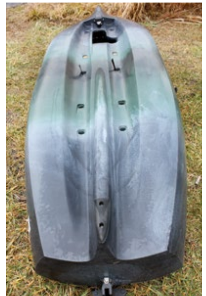
A double-U style hull provides the ultimate stability.
