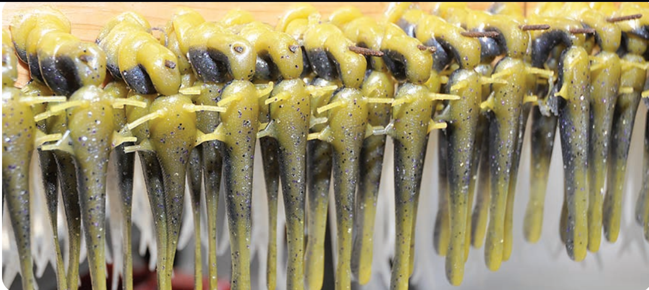
Allowing the plastic to cure for a longer period of time makes the lures more durable.
