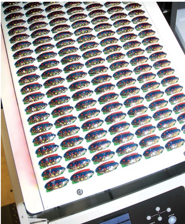
A tray of 154 buoyant lures comes out of the laser printer.
