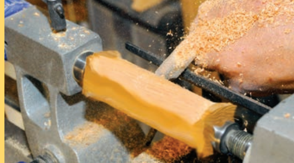
Using store-bought kiln-dried wood on the wood lathe is easier. This piece of maple is being made into a swimmer bait with a lip.
