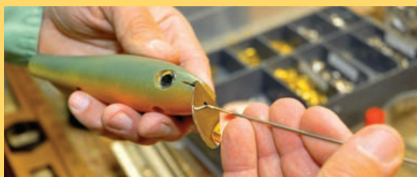
After the eyes are placed and the lip is put in position, a stainless rod is inserted and positioned to hold the hooks.
