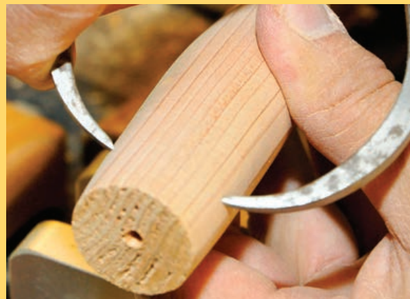
Calipers are used to mark the location of the eyes. A special drill is used to hollow the eye sockets.
