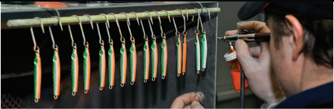
Lures are first powder coated. Then, a variety of airbrush patterns are applied. Special paint is baked on for durability.
