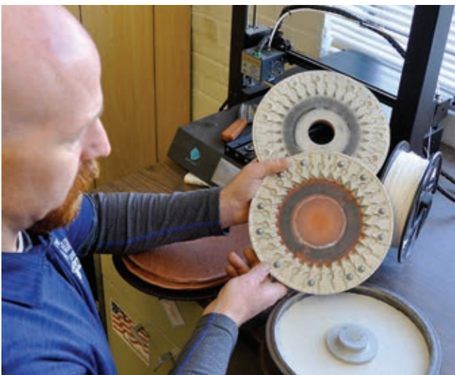
Molds are custom made in-house. Designs are first drawn in a CAD machine. Then, produced in a 3-D printer to make a master mold.
