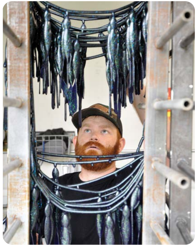
Newly formed plastic baits hang on curing racks for at least a week before packaging.
