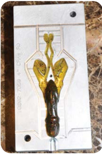
A single cavity aluminum production mold from which the final design of the Arma CRAW™ crawfish bait is produced for testing. This is the step before a production mold, with up to 100 cavities, is produced.
