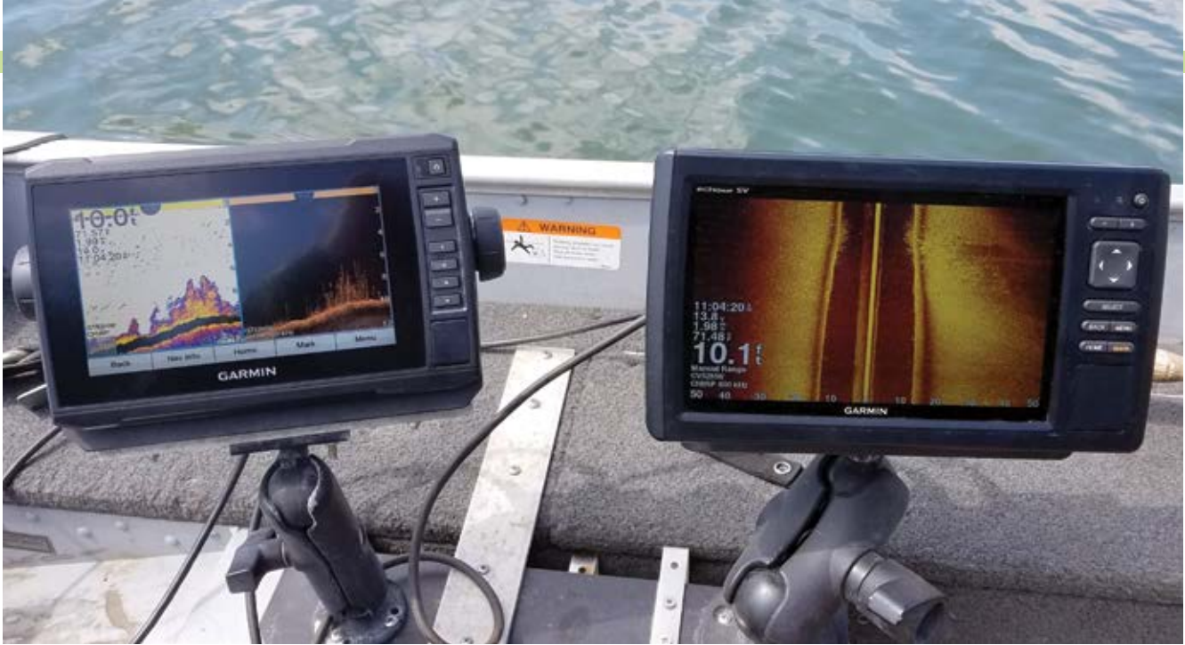
Having two side-by-side chartplotters allows the user to efficiently view charts and sonar views.
